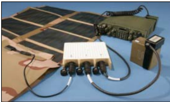
SPACES (Battery Charger)
