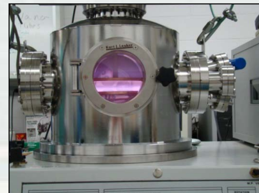
Plasma system being readied for CNT fiber irradiation experiments
