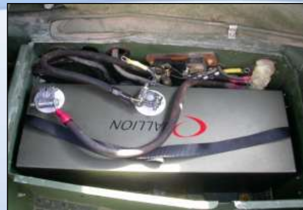
Quallion Drop-in Li-ion APU with Safety Circuit and Fuel Gauge 24V, 72Ah, 42lb
