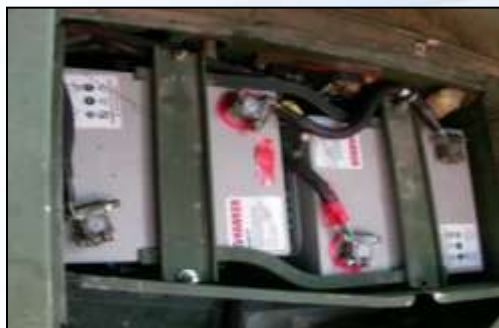
Current Lead-Acid Battery 12V x2Series, 65Ah, 59lb x2
