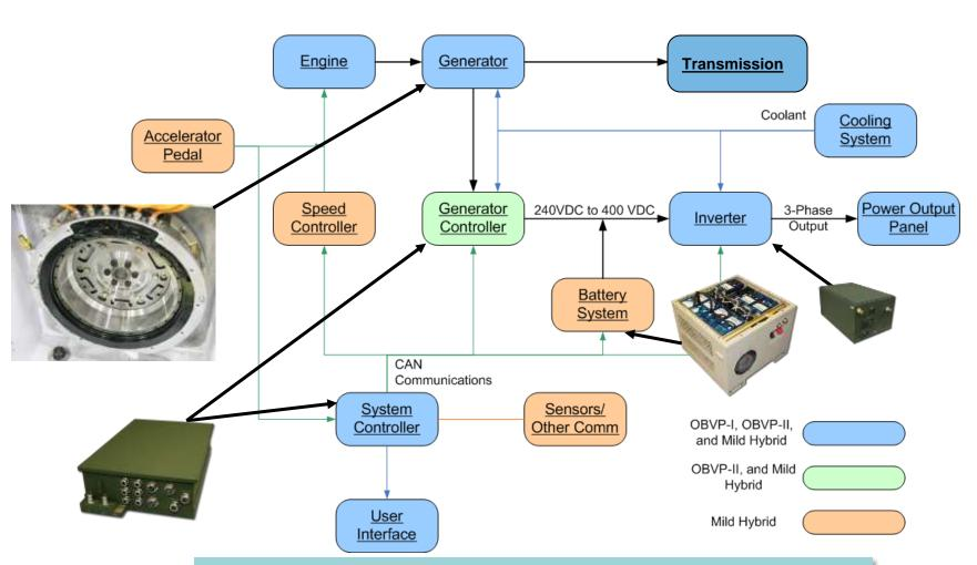
Controller will be identical to USMC HMMWV OBVP hardware developed on DRS IR&D funds. GFE Li Ion battery pack for experimental testing in GFY 11 and 12
