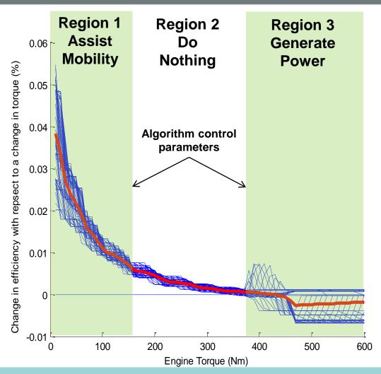
Speed does not significantly affect efficiency, the hybrid algorithm needs to monitor torque. The "rule based algorithm" will use the optimization graph to identify the 3 regions of operation as shown
