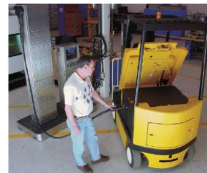
Forklifffueling - a Plug Power forklift
