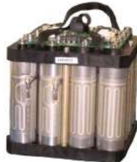
ITAS cell pack: 8S, 2P configuration
