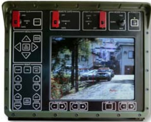
Fire Control Unit (FCU)
