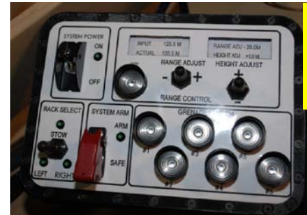
Fire Control Unit
