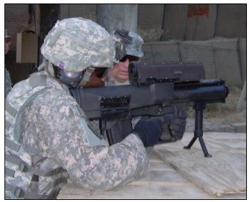
The XM25 includes an integrated, multifunctional, all environment, full-solution, day/night, target acquisition/fire control system.
