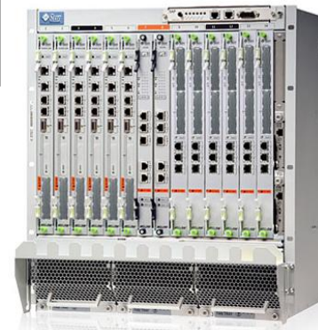
Oracle CT900 AdvancedTCA Chassis Used in SPAWAR ISNS Baseline
