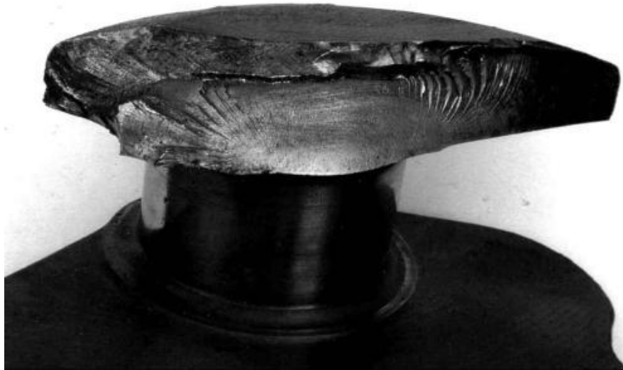
Example of crankshaft fatigue (source: Wikipedia)
