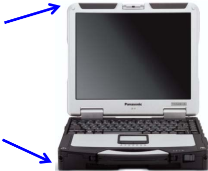
Portable Flight Line Tester for OFP load, system initialization, and diagnostics
