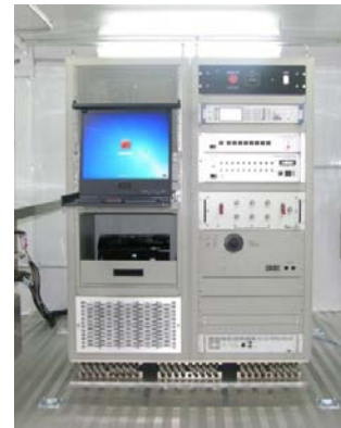
Trailer-mounted Automated System Test Set for Acceptance and Pre-Mission Testing
