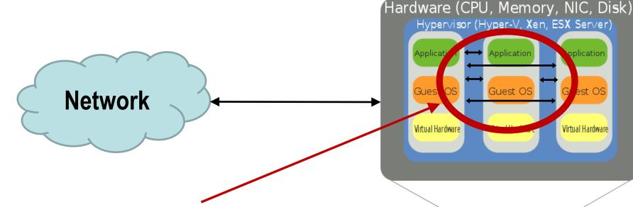
Data transferred between virtual systems hosted on the same server stack, however, never leaves the virtual environment and cannot be captured by a hardware-based collector.
