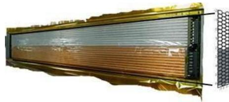
*Neutron Straws: Boron-carbide coated "straws"*
