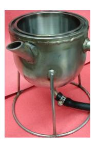
Small samples were prepared in a laboratory scale melt kettle to ensure processability. Samples underwent compatibility and safety testing
