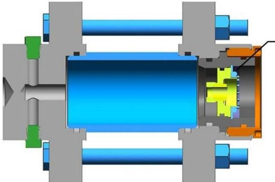
Venting Plug is held in place by snap ring. SMA phase change releases plug at ~100°C
