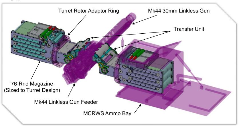
Dual feed AHS consists of two 76-Rnd magazines and two transfer units to move rounds from the magazines to the 30mm Mk44 dual feed weapon. The magazines mount to the turret rotor and rotate with the gun in elevation.
