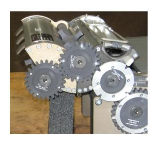
Articulating transfer unit accommodates tolerance stack-up between magazine and gun feeder.
