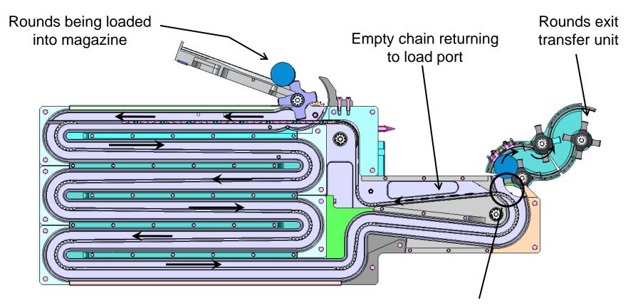
Round is transferred from chain ladder to transfer unit
