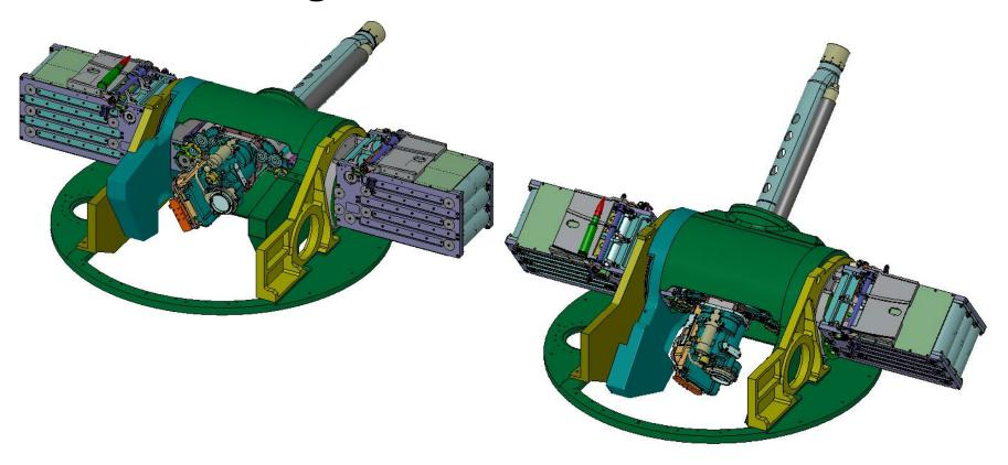
Round transfer path is simplified because of direct feet to the Gun Feeder at all elevations.
