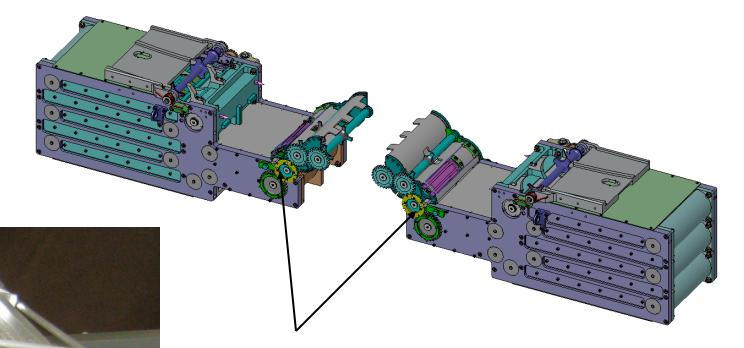
Under-armor reload ports located in both left and right transfer units. Some gun elevation is desired for optimal reload position.
