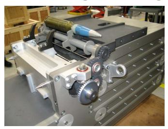
Using the gun feed-select solenoid, select the feed corresponding to the side being loaded
