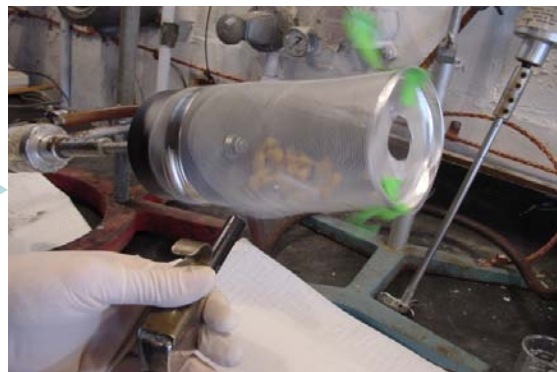
Make-shift Tumbler (pneumatic motor) + Hand Sprayer + Compressed Air
