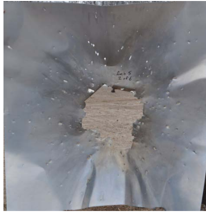
2 nd Plate (8" Behind Impact Plate) 0.040" Aluminum
