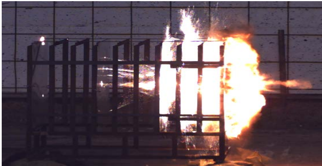
3 rd Plate (16" Behind Impact Plate) 0.040" Aluminum
