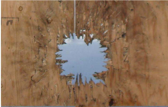
Standard LW30 M789 ~11.75" Diameter Hole
