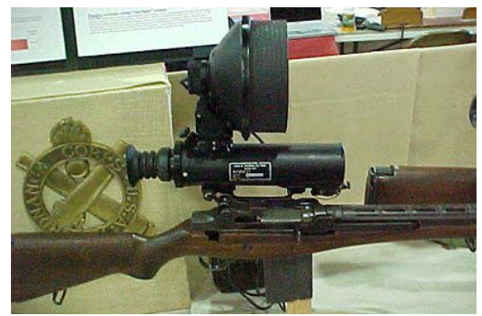
Active Infrared light source and viewing telescope
