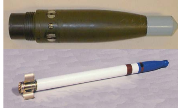
Instrumented 2.75-inch Rocket
