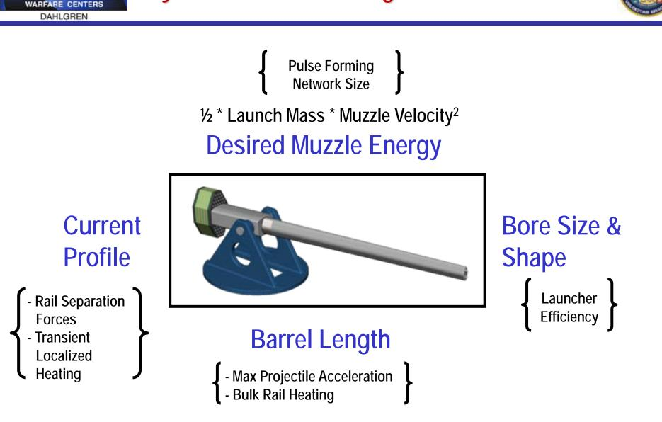
Key Parameters for Sizing a Naval EM Launcher
