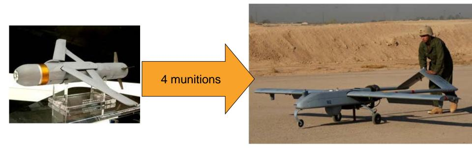
Assumed TUAS maximum payload with no degradation in ISTAR capability is 22kg
