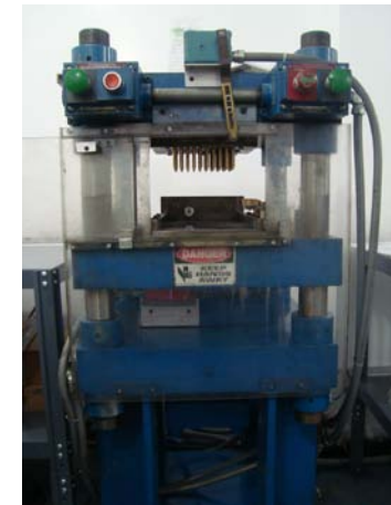
Propellant Compaction & End Cap Installation
