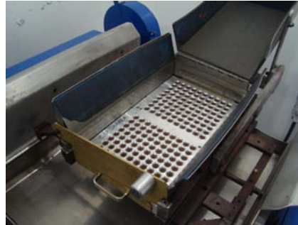
End Caps w/Bullets, Primed Case Positioned in Plates (Vibratory)
