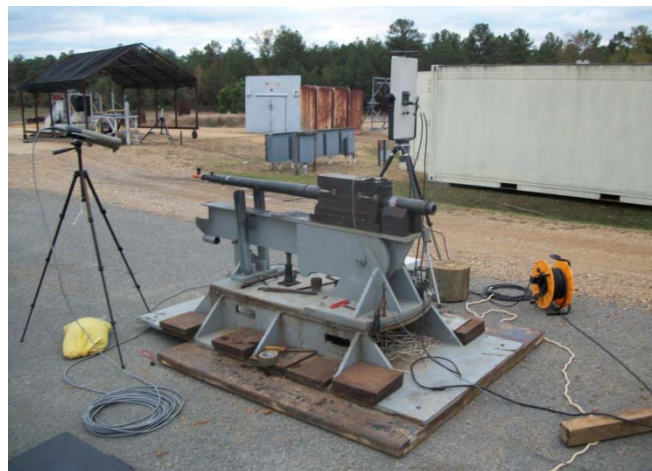
Test Barrel with radar, high speed video, and flash detector
