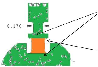
0.075" (min) hole to edge to avoid delamination problems between cover material and rigid adhesive materials
