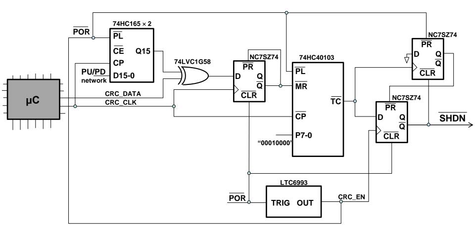
Failure of CRC verification results in shut down of 3.3 volt regulator used by the ESAD including the  $\mu$ C.
