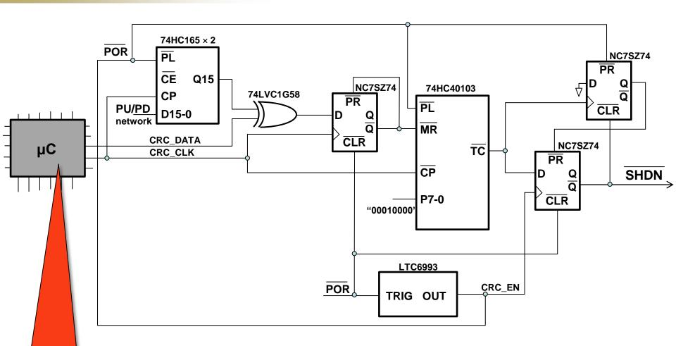
Microcontroller issues CRC data and clock pulses.
