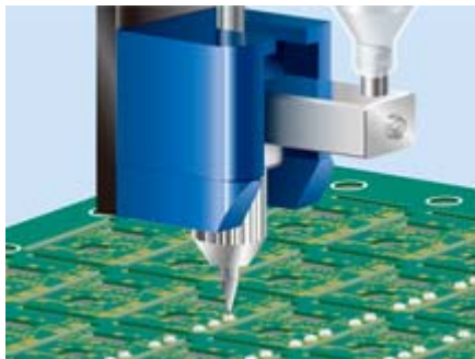
Soldering to in-vehicle substrate
