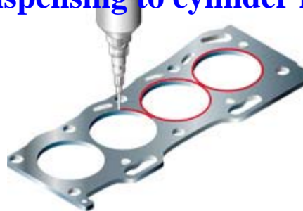
Liquid-type gasket seal-dispensing to cylinder head
