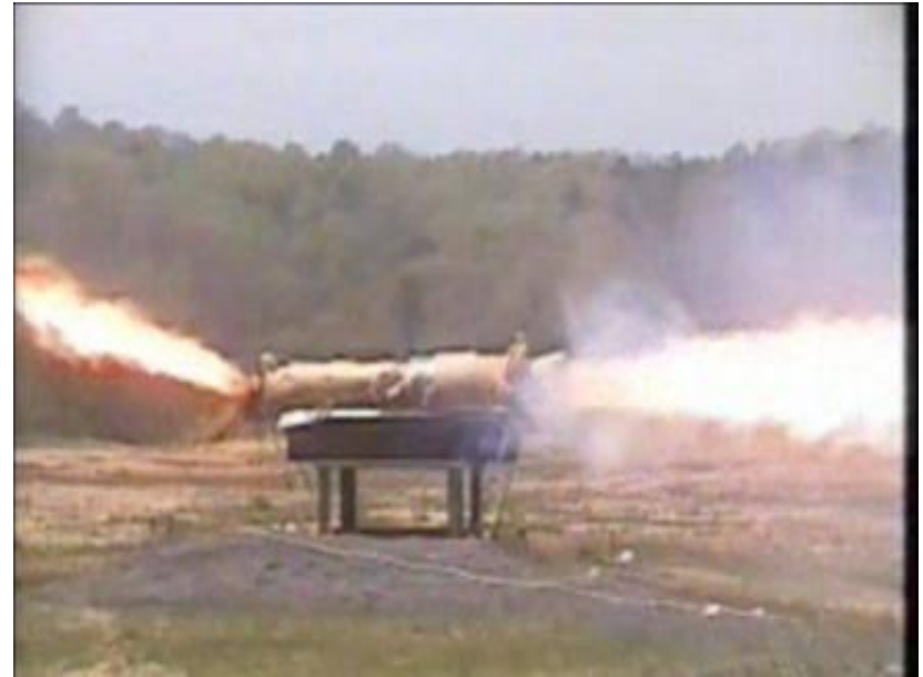
High Temperature Ignition Test (Double Venting)
