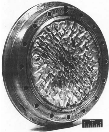
Damaged F-1 engine injector faceplate caused by combustion instability
