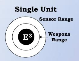
The "effective engagement envelope" will greatly expand as the shift takes place from a single warfighting unit using only local sensor and weapon resources to a system of collaborating warfighting units. The shared sensor data will enhance situational awareness; thereby extending the detection envelope and improving the reaction time of weapons deployment—which will extend the effective range of engagements.
