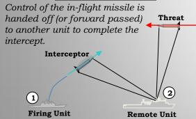
1) Firing Unit launches interceptor & passes engagement control to Remote Unit
