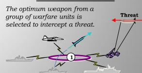
1) The best shooter is selected based on optimum engagement geometry and engageability determination. PSD can be performed in conjunction with any of the other IFC variants. PSD is, in effect, Force-centric weapon-target pairing.
