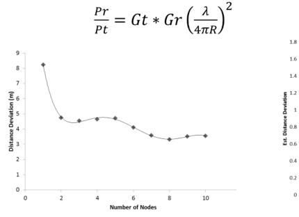
Time series collection of received power signals and hurst parameter (fading characteristics). Using statistical modeling pairing 2,3,... sensors together and using a statistical likelihood method for determining the distance of highest probability.
