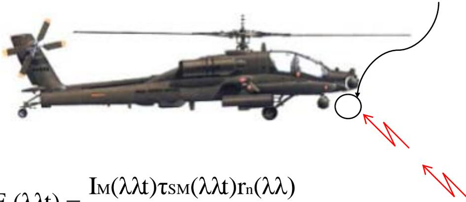
**Threat Radiant Intensity** ( $W \cdot sr^{-1}$ ) - Amount of radiation emitted from a particular area within a given solid angle in a specific direction. Spectral Radiant Intensity ( $W \cdot sr^{-1} \cdot \mu m^{-2}$ ).
