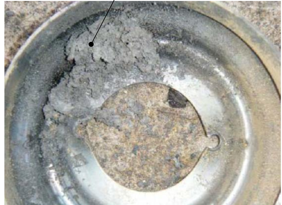
Slotted hole of front fuze liner : venting device interface
