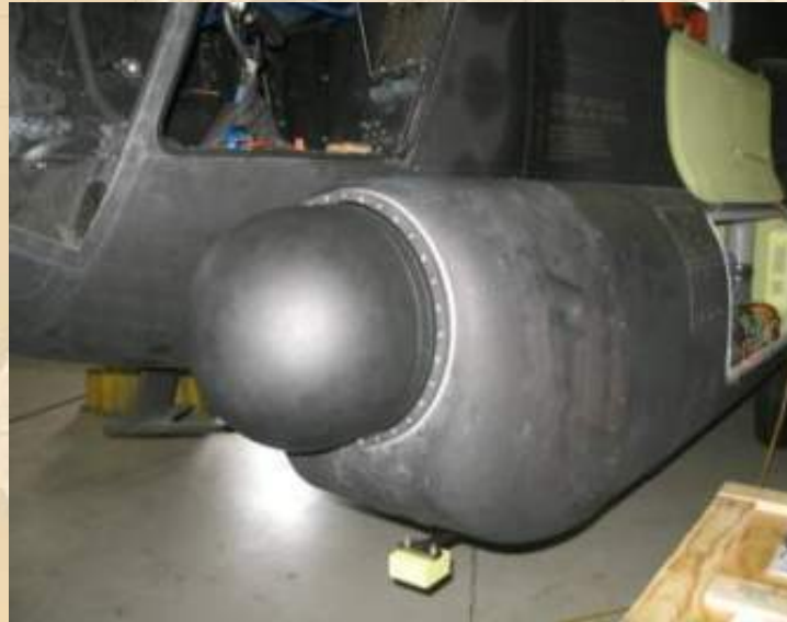
Radar Installation On MH-47G
