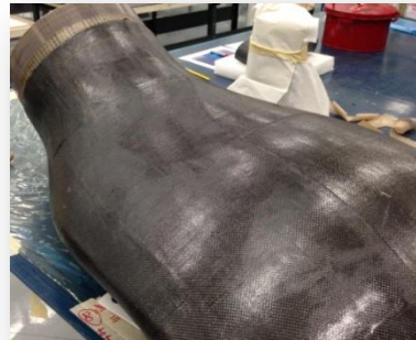
Out of Autoclave Composite Layup
