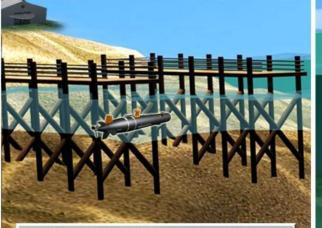
The MK 18 Mod 1 Swordfish system autonomously conducts BULS missions to provide rapid object localization for confined areas (inlets, berthing areas, between piers and pilings, confined channels and rivers) and open areas in the VSW zone (10-40 feet of sea water (FSW))
