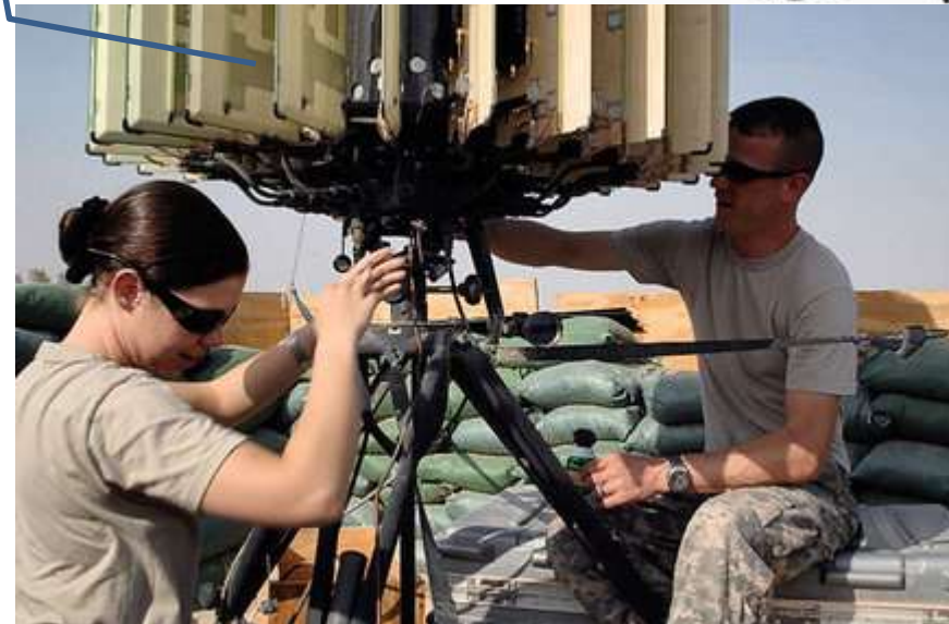
Antenna Columns (Field replaceable)
