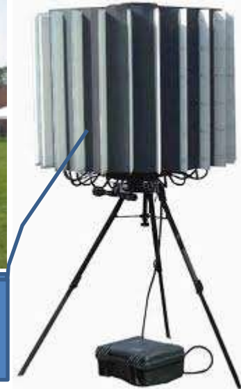
Antenna Columns (Field replaceable)
