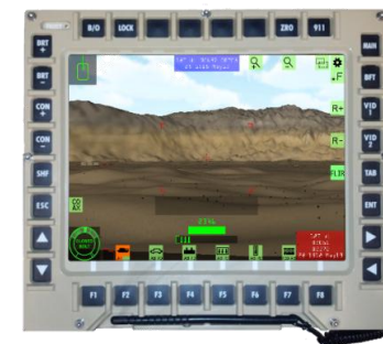
Fire Control Display / GUI
