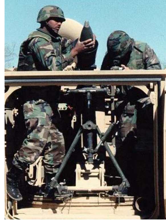
M121 120mm Heavy Mortar (Carrier) 120 mm M298 Mortar Cannon System Weight 330 lbs
