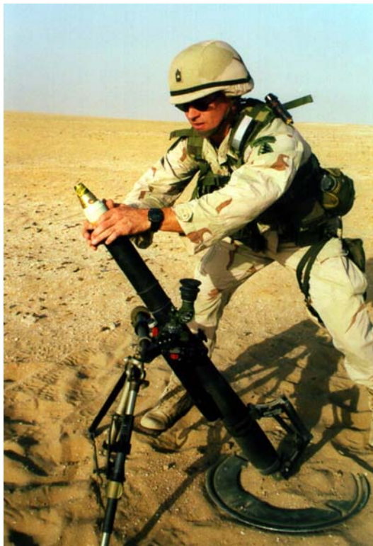
M224 60 mm Lightweight Company Mortar System 60 mm M225 Mortar Cannon System Weight: 46 lbs
