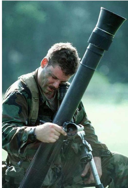
M252 81 mm Medium Extended Range Mortar 81 mm M253 Mortar Cannon System Weight 93 lbs
