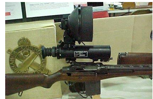
Active Infrared light source and viewing telescope
