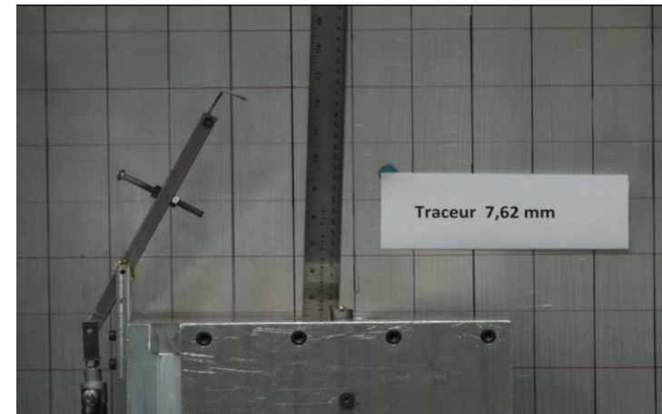
Friction initiation device, before contact
