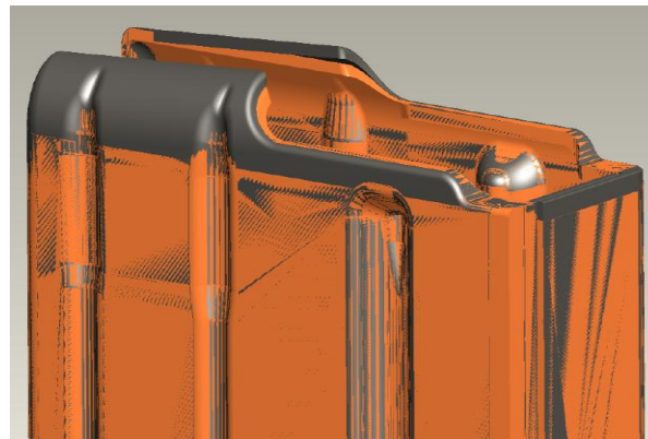
Standard magazine (orange) vs. improved magazine (grey)
