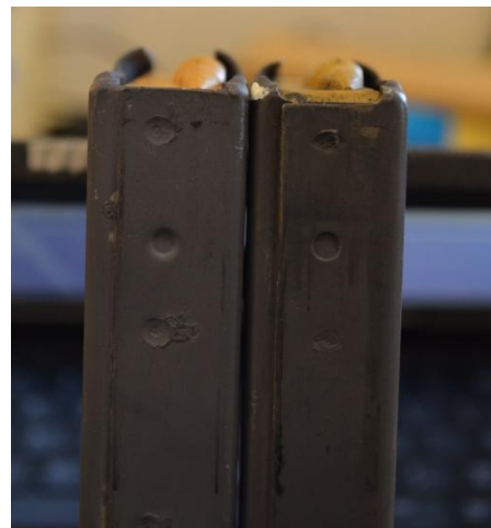
Front view of modified magazine (left) and legacy (right)
