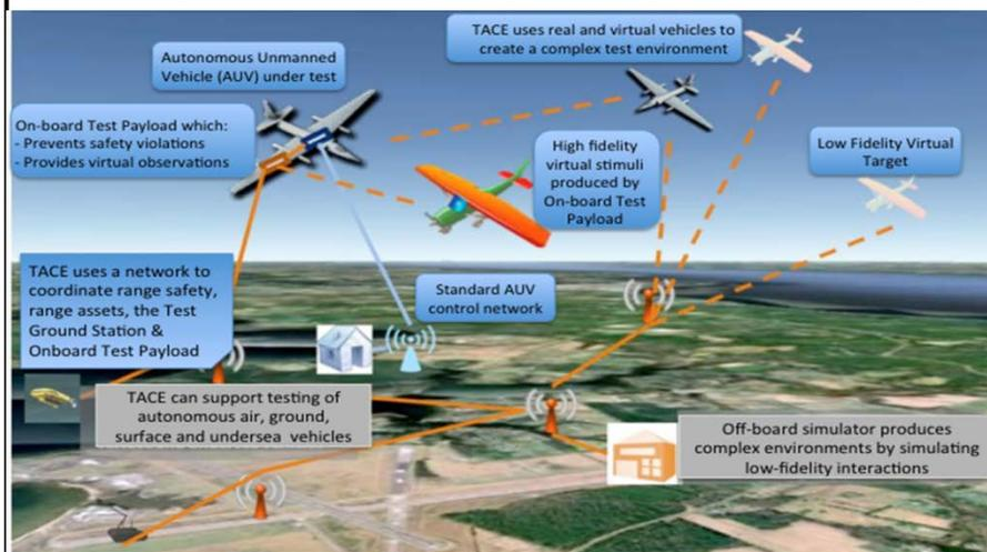
**Description:** TACE is test infrastructure that combines synthetic and actual forces to produce a realistic, real-time, interactive autonomous vehicle test environment. TACE also provides safe testing assurances via on-board safety monitoring.
