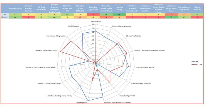
This 55 – 60 ton configuration provides improved EFP / SAIED attack protection, can carry 9 dismounts and offers some improvement relative to Legacy Platforms in the area of lethality of primary armament, weight available for growth, targeting ability, & UV protection
