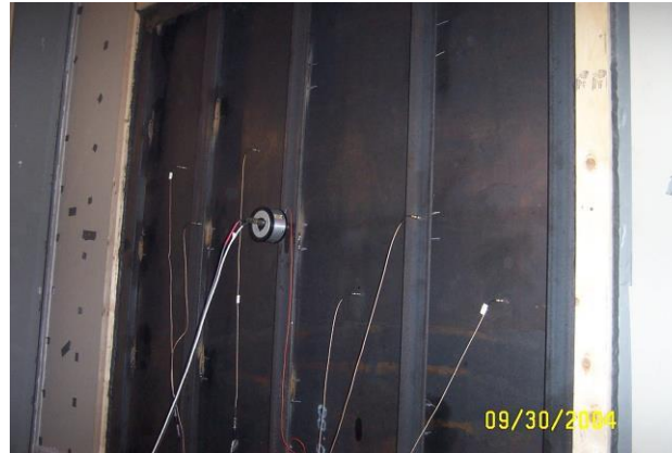
Testing Spray-on Damping
