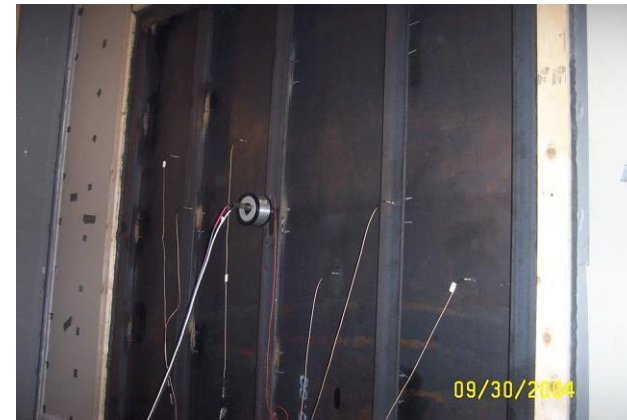
Testing Spray-on Damping
