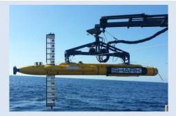
**Distributed Agile Submarine Hunting (DASH)** Extreme-depth distributed sonar for wide-area surveillance to detect and track quiet submarines
