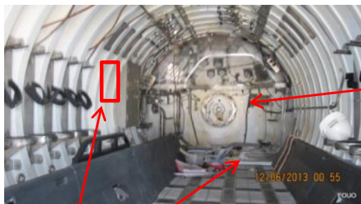
Hangar Interface Unit relocated to below deck grates
