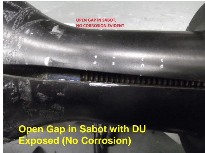
Broken Projectile Taped Together
