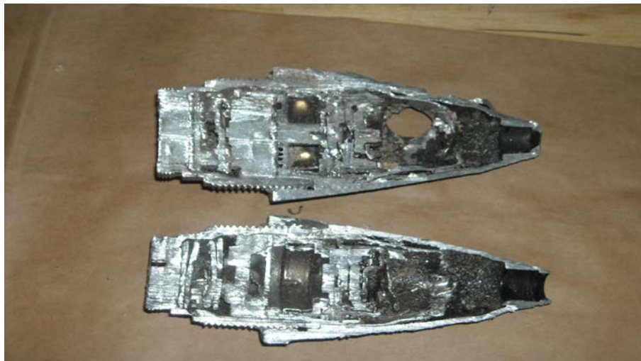
Processed 1390-N285 Mechanical Timed Fuze, cut to validate explosive free
