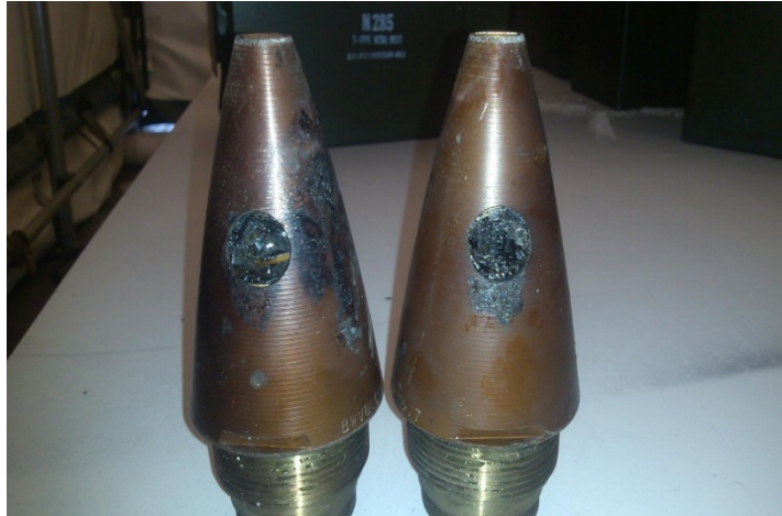
Processed 1390-N285 Mechanical Timed Fuze Post Processing
