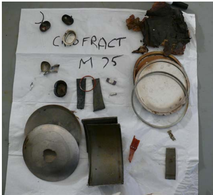
1345-K184 Cryo-fractured Anti-Tank Mine After Processing
