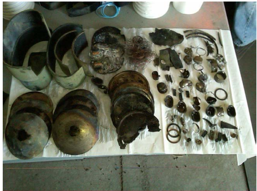
1345-K184 Cryo-fractured Anti-Tank Mine After Processing
